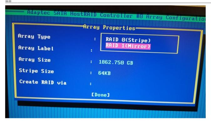
Next type in the RAID Array Label (Array Name) that you want to use, such as ARRAY1 or EXCHANGE2010 and press the Enter key.
