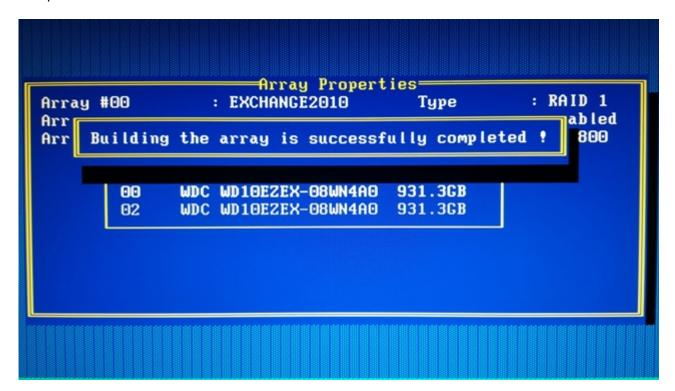
You may now press ESC, ESC to exit the Array Configuration and type Y when prompted to exit and restart or reboot the system.
