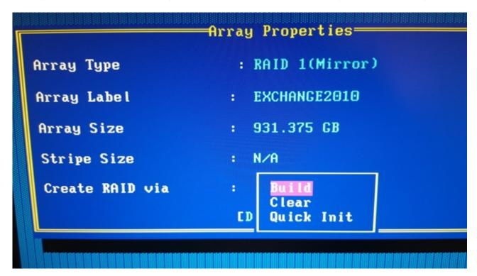
Next, press the Enter key to select "Done" at the bottom of the "Array Properties" screen.
