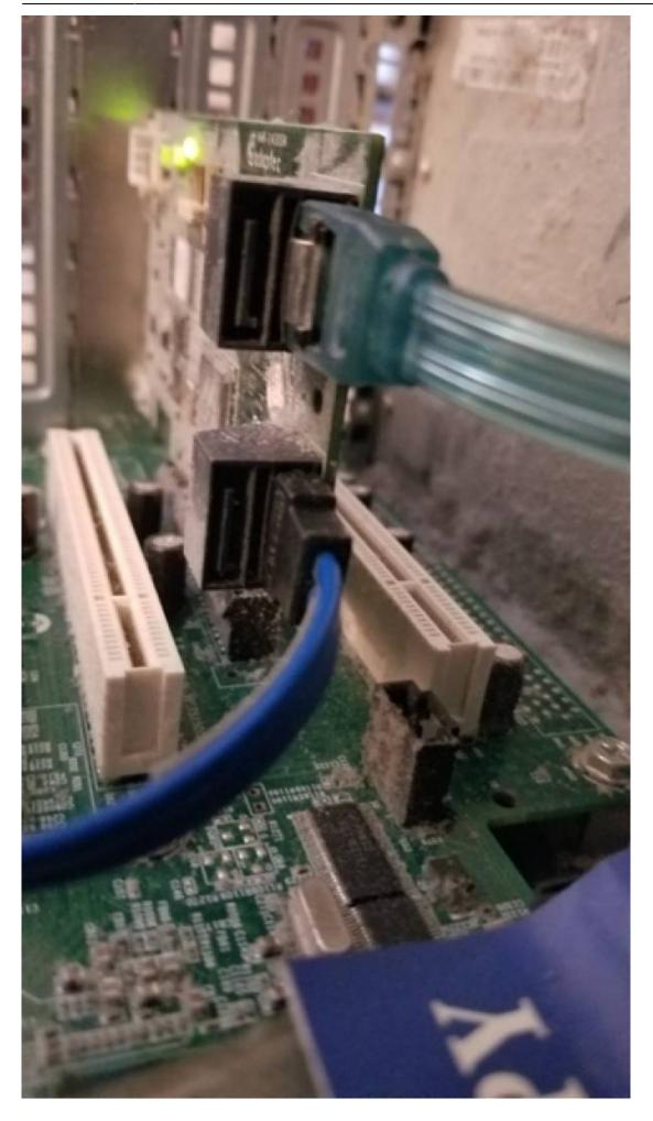
Install a brand new unused disk drive of identical size capacity or larger either on Port 1 or Port 2. I
