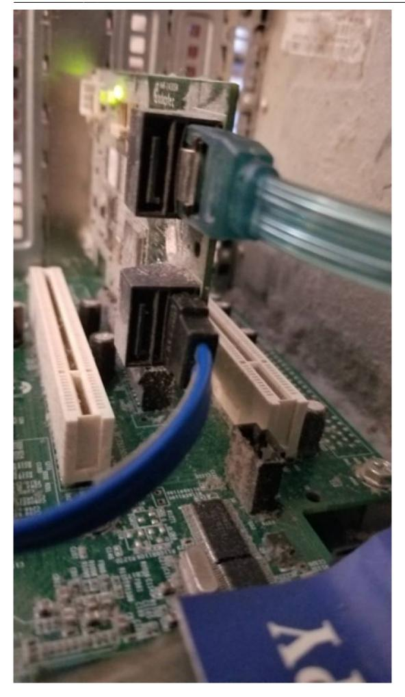
Install a brand new unused disk drive of identical size capacity or larger either on Port 1 or Port 2. I prefer port two directly above port 0. It is your choice. This will be the Target Drive of the Mirror. Then, follow the procedure to Build a RAID-1 Array.
