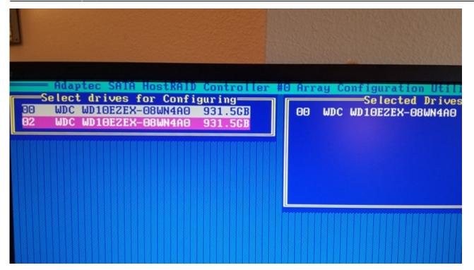
and then use the spacebar to Select Drive 02 and place it on the right side configuration, and ensure that both drives show as being selected drives on the right side of the screen.
