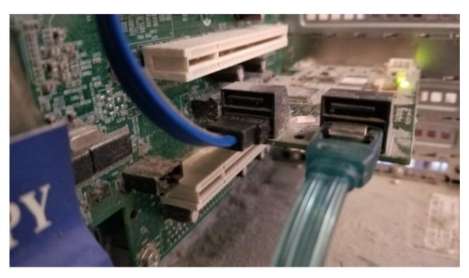
Install a brand new unused disk drive of identical size capacity or larger either on Port 1 or Port 2. I prefer port two directly above port 0. It is your choice. This will be the Target Drive of the Mirror. Then, follow the procedure to Build a RAID-1 Array.
