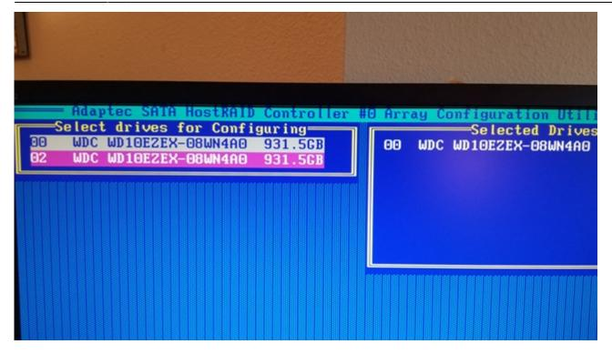
and then press the spacebar to Select Drive 02 and place it on the right side under the Selected Drives configuration, and ensure that both drives show as being selected drives on the right side of the screen.
