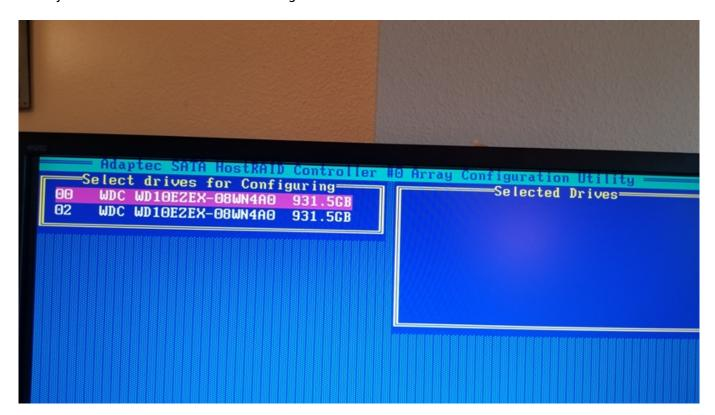
Press the space bar to select each drive on the left side of the screen to place each of them with the "Selected Drives" configuration on the right side of the screen.
