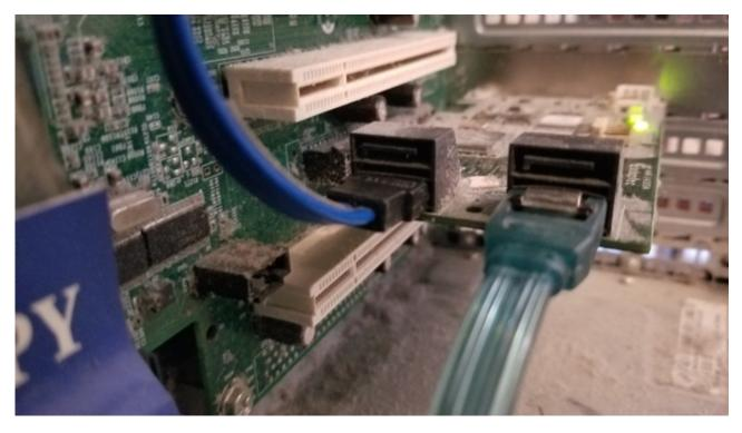
Install a brand new unused disk drive of identical size capacity or larger either on Port 1 or Port 2. I prefer port two directly above port 0. It is your choice. This will be the Target Drive of the Mirror. Then, follow the procedure to Build a RAID-1 Array.
