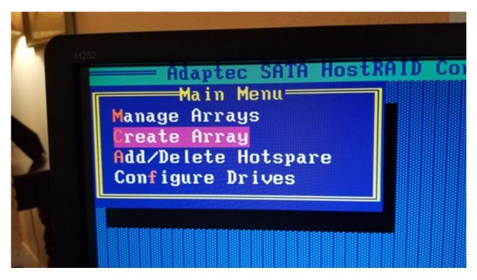
Next, press the space-bar on each of the drives in turn (on port 00 and then on port 01 or 02 as the case may be),
