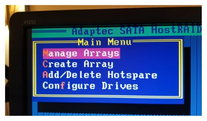
In the list of arrays, the two drives will each show as SIMPLE VOLUME, and the drive containing your operating system should be located on Port 0.
